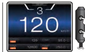
● In the checking screen, press the **Adjust+ Select buttons** to go back to the main screen.
