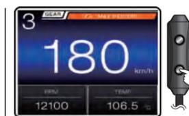
● In the Max. record screen, press the **Select button** to go back to the ODO screen.
