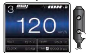
● In the Trip A screen, press the **Select button** to enter the Trip B screen.
