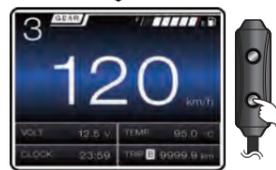
● In the Trip B screen, press the **Select button** to enter the motor oil maintenance screen.
