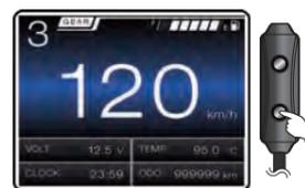
● In the ODO screen, press the **Select button** to enter the Trip A screen.
