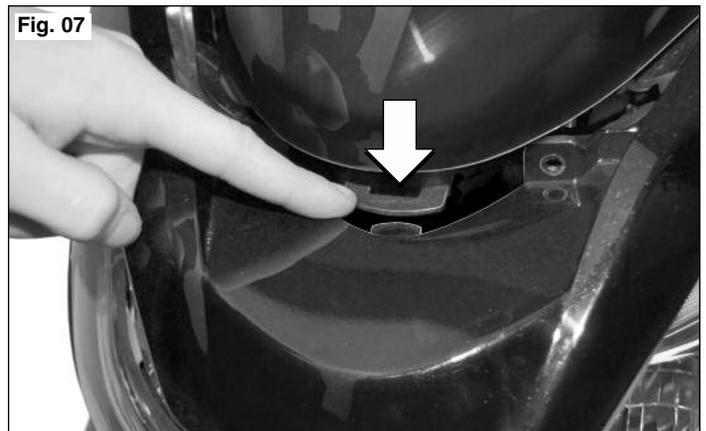
9. When the cowl is completely installed, make sure the 20x25 Dual Lock™ Fasteners under the front end are rejoined and then reinsert the two 4x16 Self-Tapping Phillips Screws under the nose of the new windscreen.
