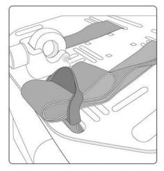
Fold the 1.5" web strap over itself, insert into and through the tension lock buckle and only snug down not fully tighten.
