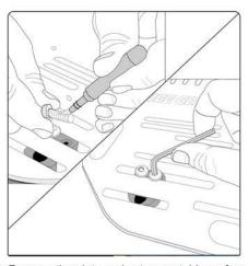
3. Remove the plate and set on a stable surface. One at a time, remove each bolt and add a small amount of the included thread lock and reinstall Tighten each bolt before installation.
