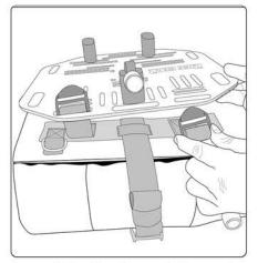
Lay saddlebag face down on table or work surface. Pull the large 2" tension lock buckles through the slots on the top of the plate.
