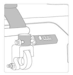
7. Slide your lock into the hole and lock into place. We find that using a gun case lock that has a minimum shaft length of 1" when closed works best for minimal movement of the lock while on the trails.
