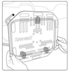
1. Hold the luggage plate up to the pannier rack to determine the optimal mounting location.
