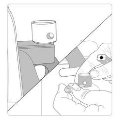
6. To use an optional lock, rotate the quick release knob until the hole of the body aligns with the slot inside the knob.
