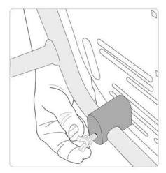
5. Once the plate is latched closed, you can slide the plate left to right to center on your rack. Once in desired position, tighten the stabilization screws located on each of the mounting feet. The plate should have little to no movement when installed correctly.
