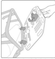
4. To attach to your rack, set the feet in place then push the top into the rack until you hear a click and the pull knob is flush with the top latch. In most cases, the latch will close automatically. Always make sure the top latch is clicked into place before each ride.
