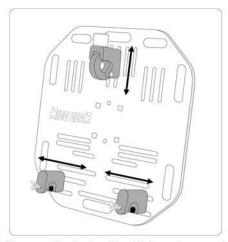
2. The mounting feet and top latch can be moved and or adjusted to find the best mounting location. Once in place, lightly tighten each bolt.
