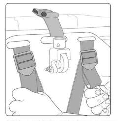
Pull down and tighten on the throw over straps using the loops made by folding the strap.
