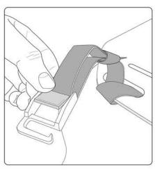
Run each of the side straps with cam buckle through side slots on the plate.
