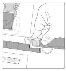
Reconnect cam buckles to one of the MOLLE loops on the bag. Center the bag and snug down the straps.
