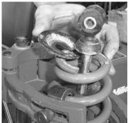
5) Once the retainer is removed, remove the spring and then remove the plastic spring collar and helper spring.
