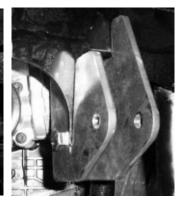
11) Connect the brackets together loosely with an M10 lock nut.
