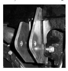
12) Connect the top of the shock to the new mount location on the newly installed lift brackets using the M10x60mm hex bolt and M10 lock nut.
