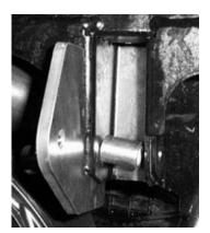
10) Using bracket ROB2 place it on the inside of the rear shock mount tab. Pushing the existing bolt from the above step all the way through.
