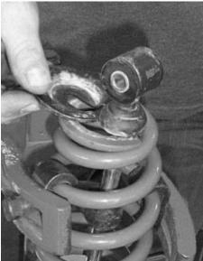
8) Starting on the drivers rear side, place bracket RIB2 on the front outside shock mount tab. It should slide into place.
