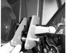
13) Connect the shock between the lift brackets and insert an M10x60mm hex bolt. Make sure to use 2 M10 washers and place 1 washer on each side of the shock eyelet. So each washer should be between the shock eyelet and the lift bracket.
