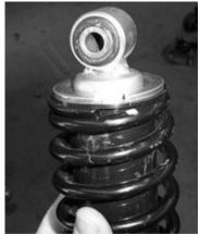
9) Use bracket FRB1 (this is if you start installation on the front right) and place it on the rear facing side of the shock mount.
