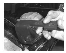
6) Install the brackets on the outside next to the shock mount and loosely fasten them together. Make sure to follow the correct orientation described in step 4. Therefore, after placing RCB2 on the frame, place RTB2 in the middle, and RSB2 on the bottom.
