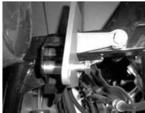
12) Use bracket FOB2 and place it on the outside of the shock mount tab onto the bolt just installed. Fasten the bolt with an M10 lock nut.
