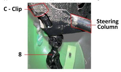
**Step 5** Reinstall remaining stock C-Clip to Upper Shaft (8).
