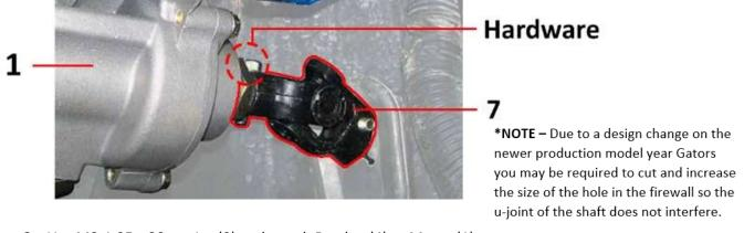
**Step 3** Use M8-1.25 x 20mm Lg. (9) and attach Bracket (4) to Motor (1).
