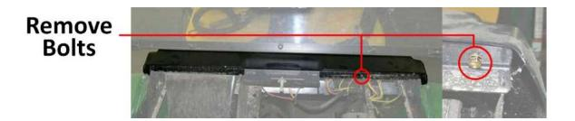
**Step 5** Remove two Bolts from Glove Box, and one Bolt from Steering Cover; Remove Dash.
