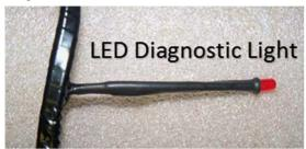
If there is a malfunction with an electronic part, the system will create a code to identify the problem. Each fault codes displays by a series of flashes with a fault light. Fault codes show with a light.
