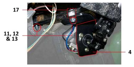
Step 7 Install Stabilizer Bracket (5) to Mounting Bracket (4) with M6-1.0 x 20mm Lg. (14), M6 Flat Washers (15), and M6-1.0 Nylock Nut (16). Secure opposite end to slot, located in Frame, with M6-1.0 x 20mm Lg. (14), M6 Flat Washers (15), and M6-1.0 Nylock Nut (16).
