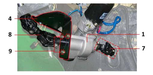
**Note** — If there are two #4 BOM mounting brackets in your kit as seen below — the correct bracket to use for your installation is the bracket circled #1 below which has no offset on the flange tab.
