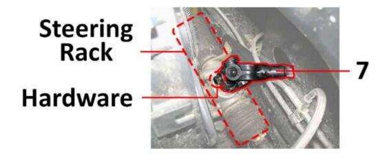
**Step 2** Attach Motor (1) to Lower Shaft (7) with supplied hardware.
