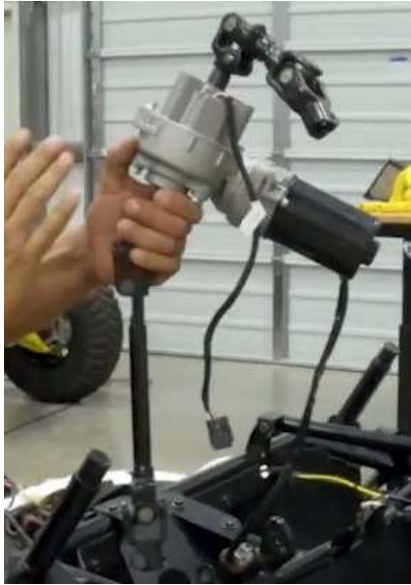
Pre-assembled with short shaft, long shaft and motor
