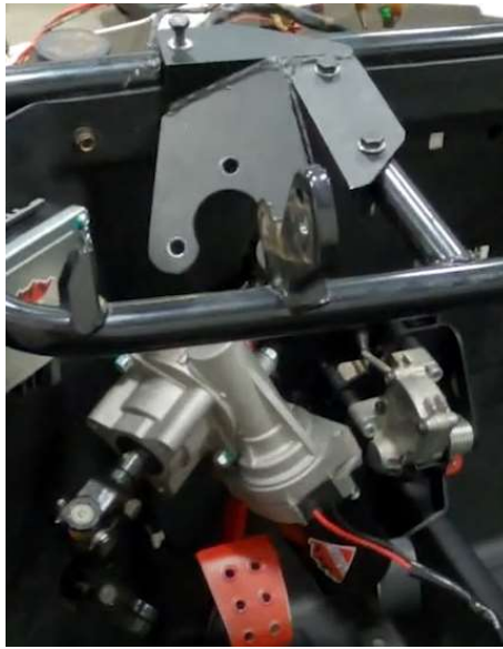
Test fit unit inside vehicle to see shaft position against firewall, this will need to be cut
