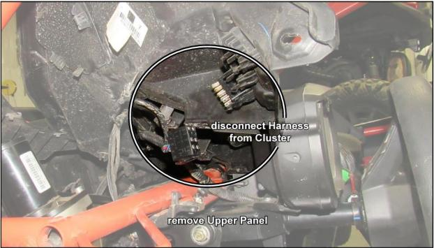
**Step 3:** Remove the bolts and nuts as shown on the pictures. Make sure to make a note and keep them in the same order you removed them so they can be installed in the correct orientation.
