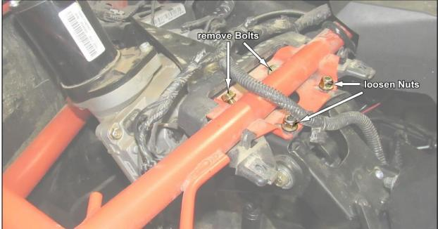
**Step 4:** Unplug all the connections on the motor. Protect the connections with tape to keep the water out.
