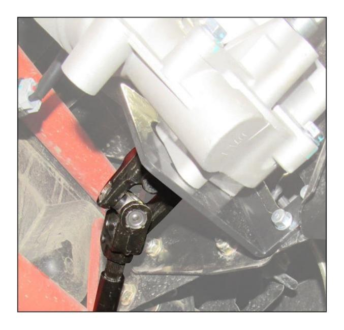
**Step 12:** Install the upper shaft into the steering support and secure with snap ring.
