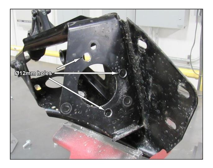
Method B (2018+): mount bracket 1 directly onto the frame with the M8x25mm flange bolts and M8 nuts.
