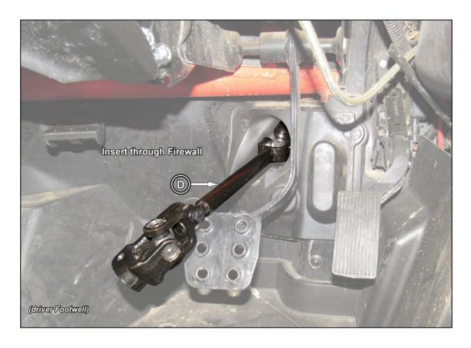
**Step 11:** Install and secure the lower shaft and bracket 1 onto the motor with the M10x20mm flange bolts as the picture shown.
