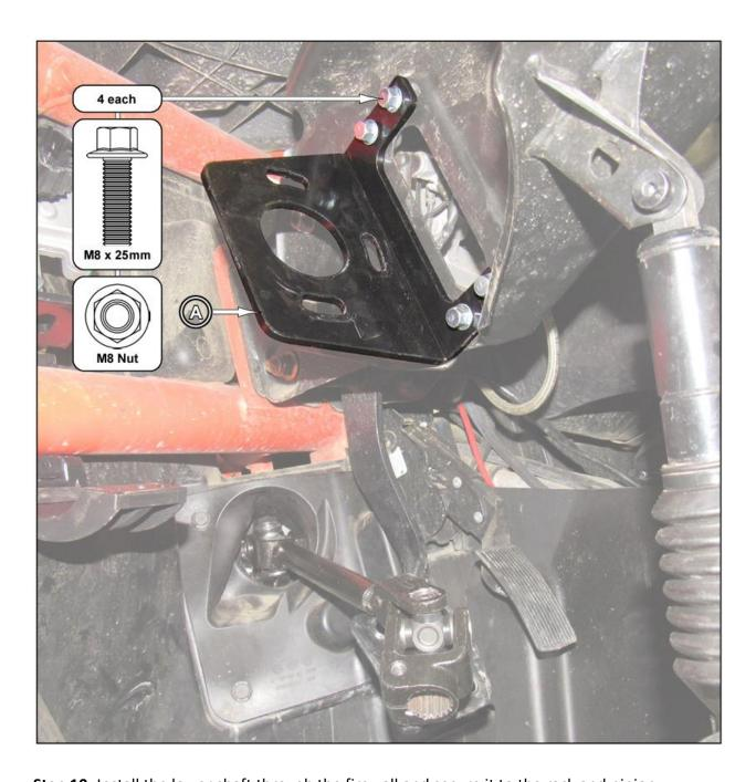
**Step 10:** Install the lower shaft through the firewall and secure it to the rack and pinion.
