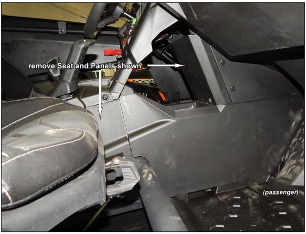
**Step 2:** Loosen the upper panel and disconnect the harness from cluster. Then remove the upper panel.
