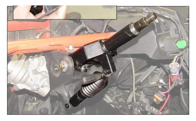
**Step 14:** Secure the steering support and the tilt adjustor and reinstall the steering wheel.
