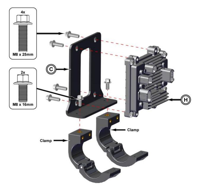
**Step 16:** Secure the bracket 3 assembly onto the cage.
