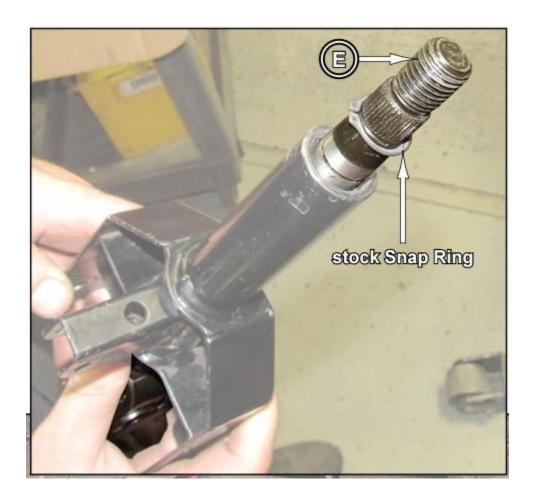
**Step 13:** Secure the upper shaft to the motor.
