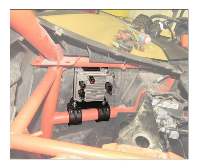
Step 17: Connect the wiring harness to ECU following wiring procedures.
