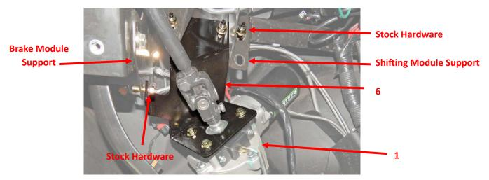
**Step 6** Install the hardware in the image below through the brake module support. (The upper shaft (8) is not shown in the image for clarity purposes.)
