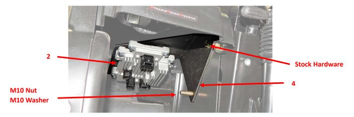
**Step 8** Tighten all hardware completely and reinstall the dash, steering wheel, and all other required stock components.
