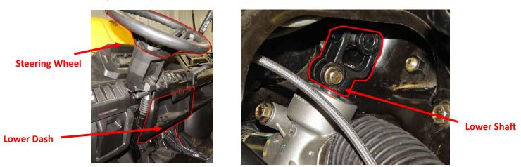
Step 2 Remove the steering box cover, steering column, and the adjustment cylinder
