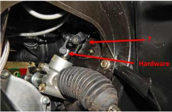
**Step 2** Place the motor mount (6) onto the shifting module support studs, then reinstall the shifting module support.
