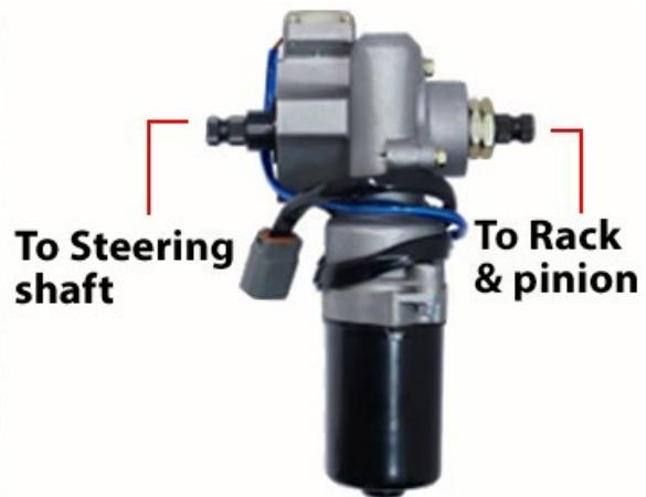
Fabricate upper steering shaft using supplied upper shaft and OE upper shaft. Make sure the length is does not differ from original OE shaft. Insert into steering column using factory spacers and mount onto motor
