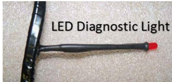
If there is a malfunction with an electronic part, the system will create a code to identify the problem. Each fault codes displays by a series of flashes with a fault light. Fault codes show with a light.
