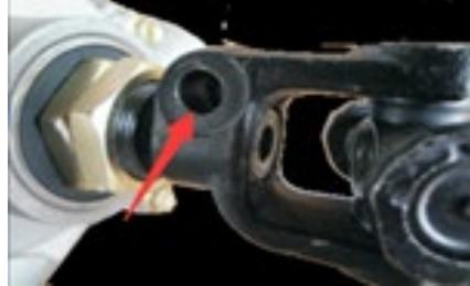
11. When installing the shaft, please adjust the bracket to make sure u-joint is not at large angle otherwise there may be interference issues.
