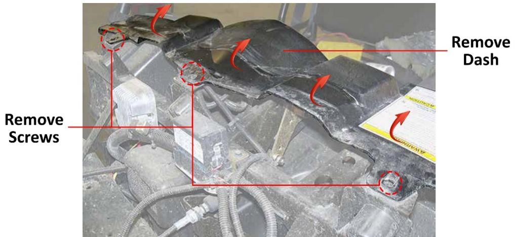
**Step 3** Remove any wire harness' that are connected to dash.
