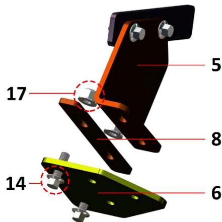
**Step 5** Install motor bracket (4) to mounting plate (6) with bolt (14) and nut (17). Use two bolts (15) and nuts (17) to join motor bracket (4), mounting plate (6), and mounting bracket (5) together.
