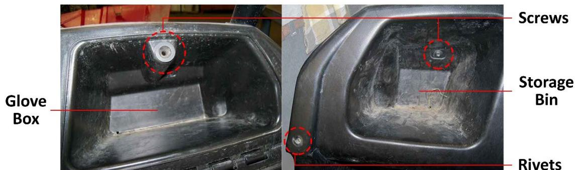
**Step 6** Remove plastic rivets where dash installs to firewall.
