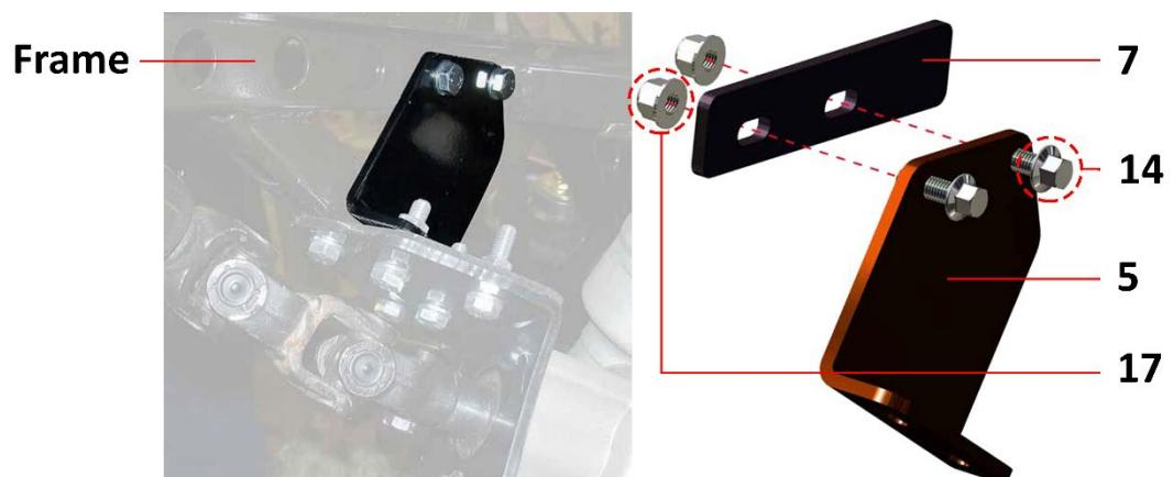
**Step 4** Install lower pinch plate (8) to inside of frame and mounting plate (6) to mounting bracket (5). Secure with bolt (14) and nuts (17).
