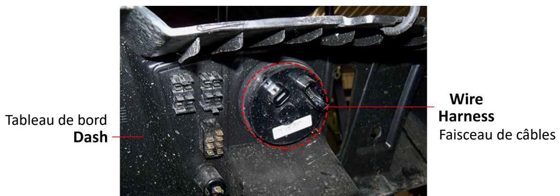
**Step 16** Remove parking brake knob and ignition switch.
