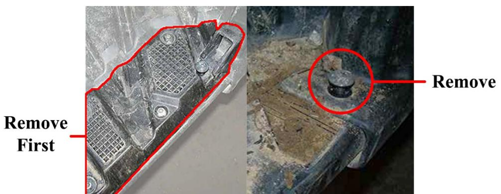
**Step 11** From driver side fender well, remove inner panel.
